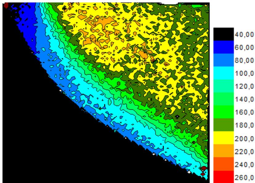
**Figure 4: EBT2 film dosimetric distribution in cGy.**
