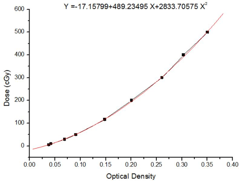
**Figure 3: Calibration curve obtained in the red channel.**
