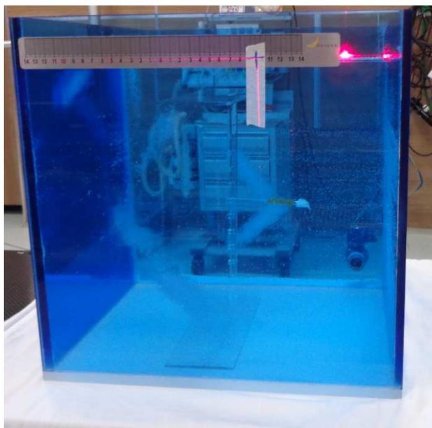
**Figure 2. Water phantom and support used in the calibration of the films.**
