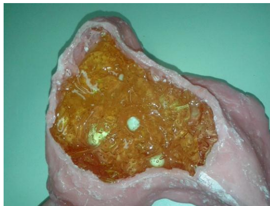
Figure 2. Representation the phantom with conductive gel and Styrofoam balls.
