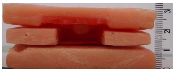
Figure 4 Representation of the stacking order of acrylic plates was used during the tests with the phantom.
