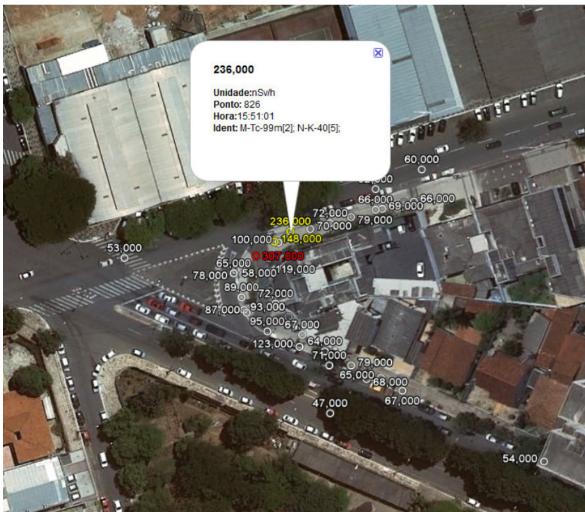
Figure 7. Identification of the presence Tc-99 from a Medical facility at Goiânia-Brazil. The stamp shows time, date and file identification of the spectra.
