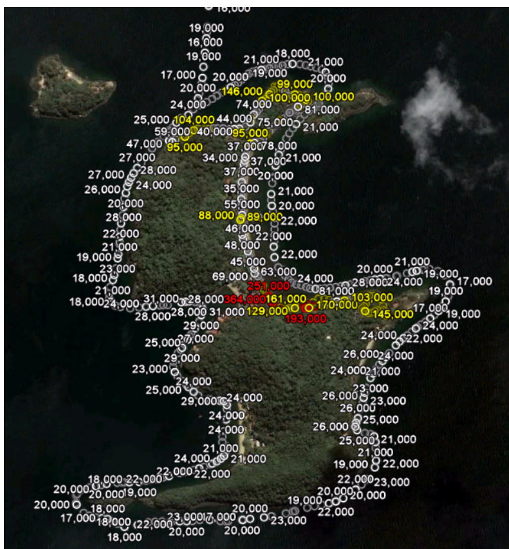
Figure 4. Survey over Itaguai Bay and Martin Island. The external perimeter was done by trawler, near the shore. In the middle of the island the Atas Scanner was used as manborne system. The high values are due decorative stones in fences and houses.
