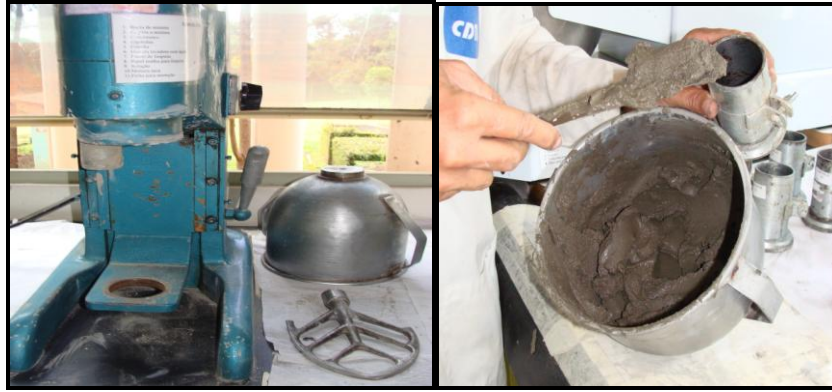
Figure 1. Mixer and cement paste containing simulated waste and chemical additive
