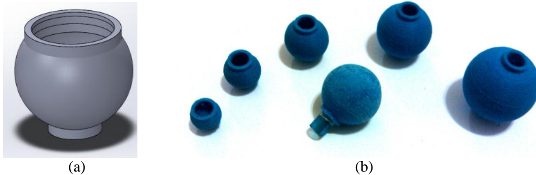
Figure 3. 3D model of a hollow sphere (a) and the built hollow spheres (b).
