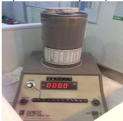
FIGURE 1: Activimeter model CRC-7 - Capintec. Photo kindly given by the Center of Nuclear Medicine of Pernambuco (CEMUPE) in Brazil.
