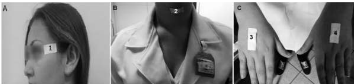
Figure 1. A) The MCP TLDs (envelop 1) are positioned near the assistant's left eye; B) The MCP TLDs (envelop 2) are positioned on the assistant's neck (under the lead protector); C) The MCP TLDs (envelops 3 and 4) are positioned on the assistant's hands.
