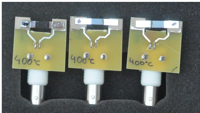
**Figure 2 – ZnO nanofilms soldered to printed circuit board with BNC connector.**
