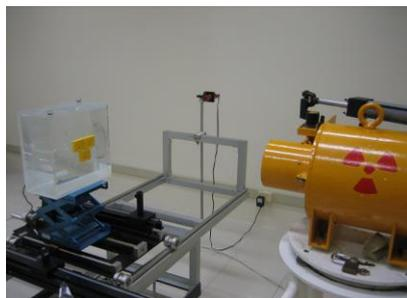
**Figura 2: Experimental arrangement 1 - slab phantom.**
