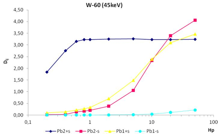
**Figure 3:  $D_{ij}$  as a function of  $H_P(10)$  in the filter to lead the energy of 45 keV - more sensitive and less sensitive emulsion, for the arrangements 1 and 2.**
