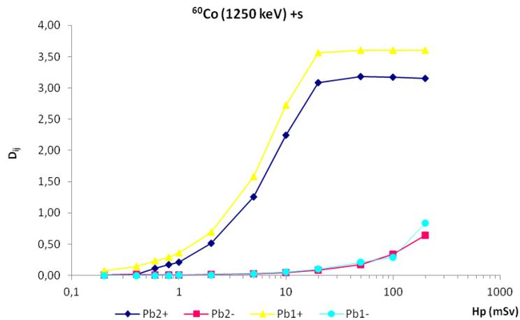
**Figure 4:  $D_{ij}$  as a function of  $H_P(10)$  in the lead filter to the energy 1250 KeV - more sensitive and less sensitive emulsion, for the arrangements 1 and 2.**
